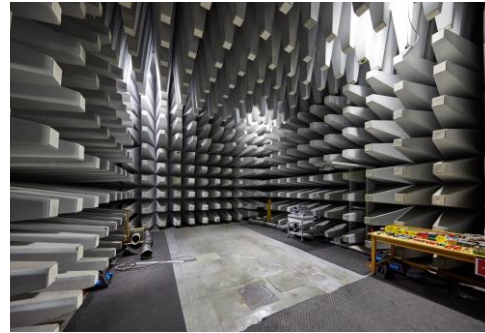
Semi anechoic chamber for vehicles Emission received by onboard antennas
