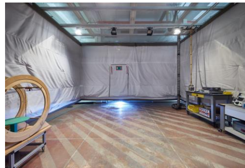
EM-Field screened tent Customer specific tests
